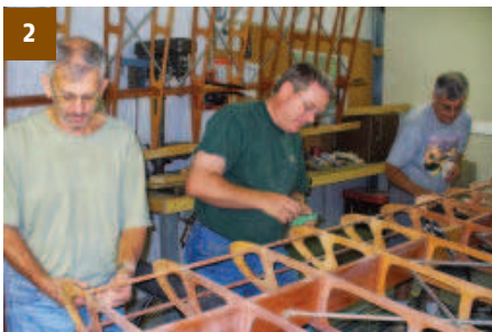
1) Left wing during repairs to wood.
