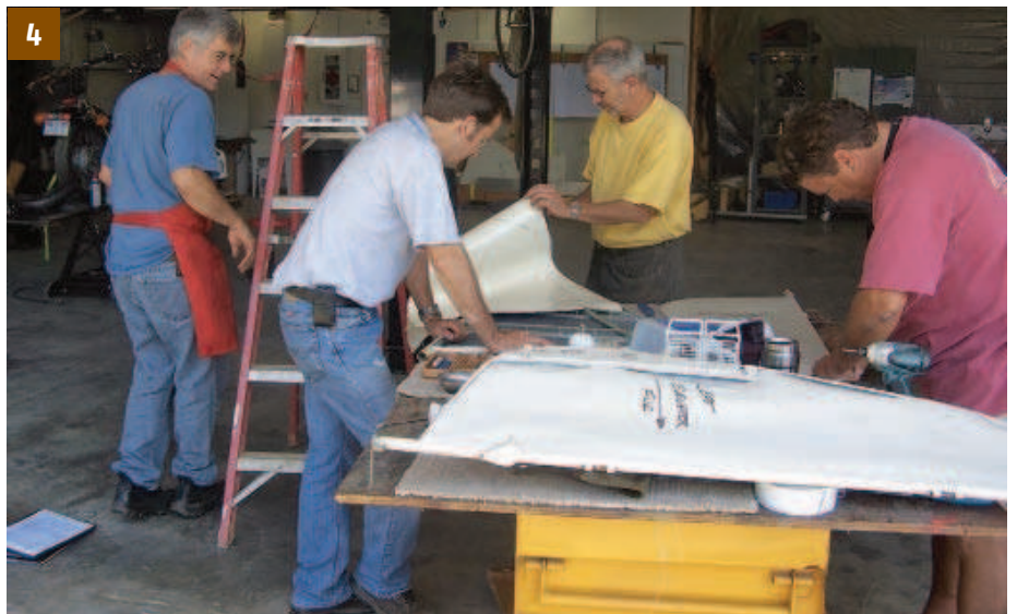
2) (L to R) Joel McLaughlin, Andy Thomson, and Terry Gardner add plywood doublers to rib leading edges to repair minor damage.
