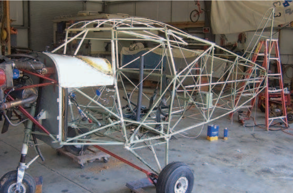
The Skycoupe fuselage, just after removal of old fabric.
